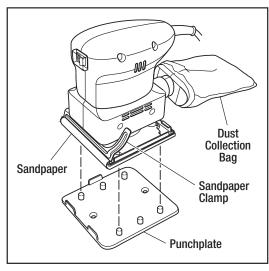
FIGURE 4. USING THE SANDPAPER PUNCHPLATE
